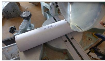
You can cut the tube to 9 1/2 " with a chop saw or razor blade.
