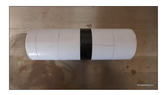
I covered my tube with white duct tape to make it last longer and protect it from water. I used white duct tape so it would not absorb solar radiation and get warm before use. A cool Macroscope will allow you to look at unaltered snow crystals longer. I put one piece of black tape on the tube so it would be easy to see in the snow.
