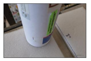
Trace the tube on the outside diameter. Bigger is better so it will fit snuggly in the end.
