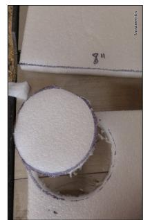
Cut the end piece out with a sharp blade.
