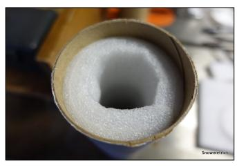
Cut a rectangular piece of foam, roll it, and insert it into the tube. Push it in a short distance so the end piece and cap will fit too.
