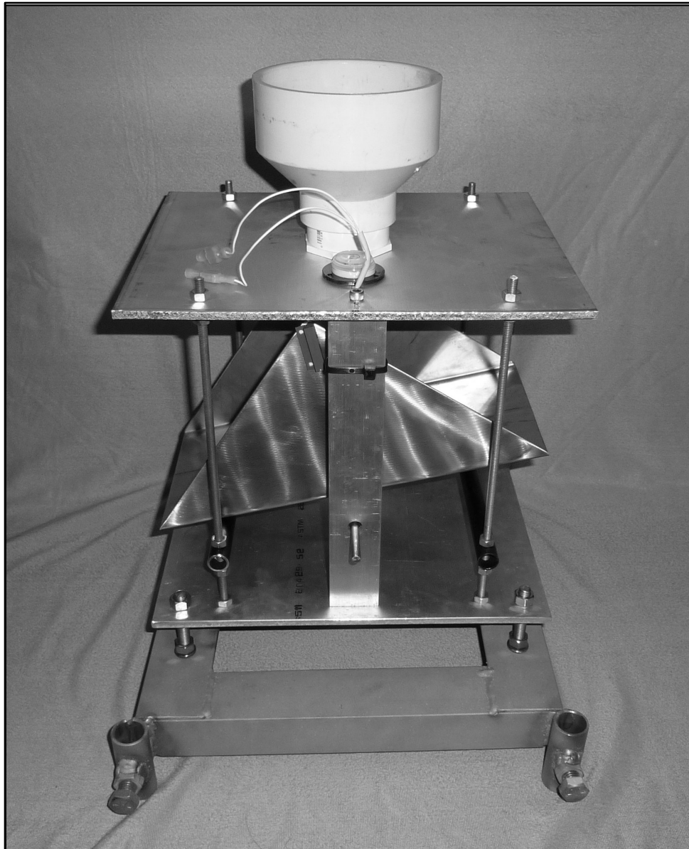
Figure 8. Final tipping bucket assembly with funnel unit and ground plate attached.
