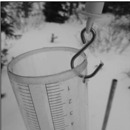
← 9. Place the scale hook in the hole on the tube.
